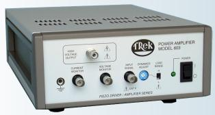
The Trek Model 603 is a high-voltage DC power amplifier/piezo driver designed to provide precise control of output voltages in bipolar or unipolar ranges that are customer specified within a range of available settings. The instrument achieves the accurate output responses and high slew rates demanded by reactive loads by utilizing a four-quadrant active output stage that sinks or sources current into reactive or resistive loads.
