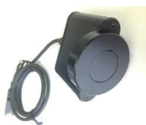
Non-destructive probe Meas.Spot : φ25 mm
