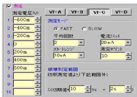
Conditions to measure V-I curve
