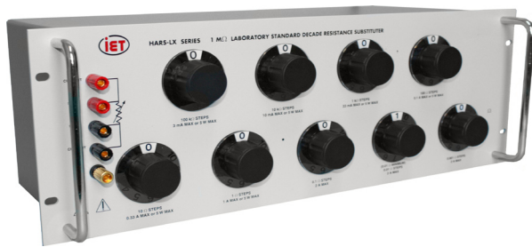
Nine-decade Model with 1 mΩ resolution
