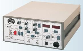
The Trek Model 615-10 is a precision high voltage AC/DC generator and amplifier system used in a broad range of R&D and production applications. In the constant voltage mode, the 615-10 generates constant amplitude waveforms with or without DC bias. In the constant current mode, it generates constant amplitude AC current waveforms, with or without DC bias and in amplifier mode, an analog voltage input connector is provided to apply external AC or DC signals.
