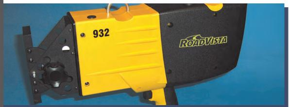
The <u>RoadVista Model 932</u> is a handheld retroreflectometer designed for use in the field, laboratory or QA/QC environment. It is designed to fully characterize the retroreflection (RA) and retroreflected night-time (CIE1931xy) color of road signs, high visibility safety clothing and other materials.
