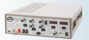
The Trek Model 615A-1 and the Model 615-3 are precision highvoltage AC/DC generators that can be used in constant voltage, constant current or external amplifier mode. They are specifically designed to simultaneously provide the AC and DC operating potentials required to operate/control an electrostatic charger roller and offer features such as four-quadrant output, high rejection of load current noise and three wave output shapes.
