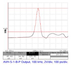
The AVH series of low jitter, high output amplitude impulse generators provides pulse widths (measured at the 20% rise time point) in the range of 130 ps to 2 ns, amplitudes as high as 100 Volts, with pulse repetition frequencies to 1 MHz.
