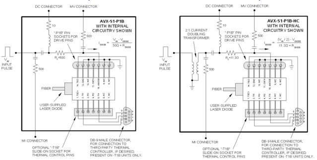
The exact pin configuration of the diode package must be specified at the time of ordering, so that a suitable socket can be provided. The above circuits illustrate one common configuration, which requires a positive pulser. See the AVX-S1 and AVX-S1-HC datasheets (<a href="http://www.avtechpulse.com/laser-bias/avx-s1">http://www.avtechpulse.com/laser-bias/avx-s1</a>) for more information and for examples of packages that can be accommodated.
