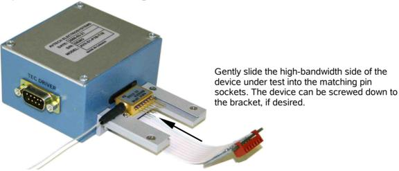
Step 3 - Install the Slide-On Socket on the Low-Bandwidth Pins
