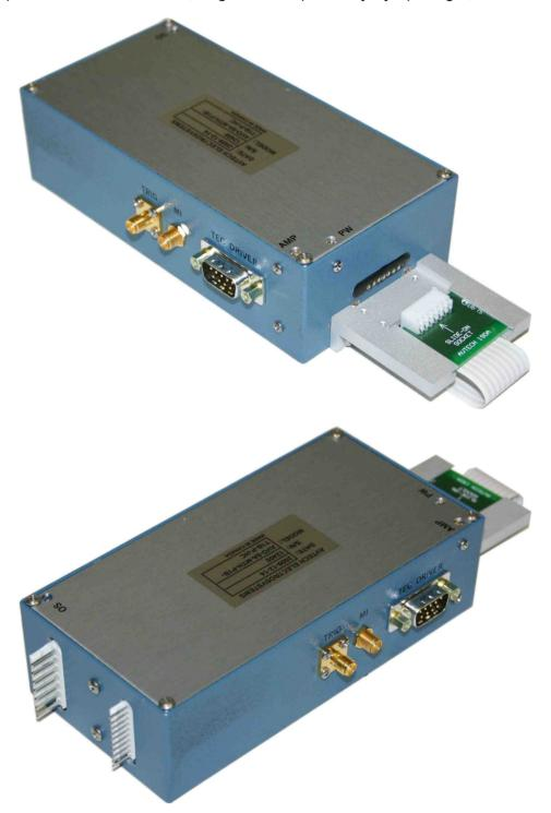
The basic dimensions of the blue module shown in the photo (excluding the connectors and brackets) are 1.67"  $\times$  3"  $\times$  6", or 42.4  $\times$  76.2  $\times$  152.4 mm.
