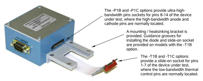
Step 2 - Insert the Diode into the High-Bandwidth Pin Sockets
