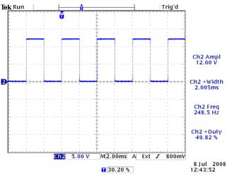
AVR-9A-B output, 12V, 250 Hz, 50% duty cycle, into  $10\Omega$
