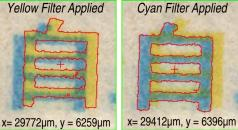
Color registration: Centroids are offset in x by 360μm and in y by 137μm.
