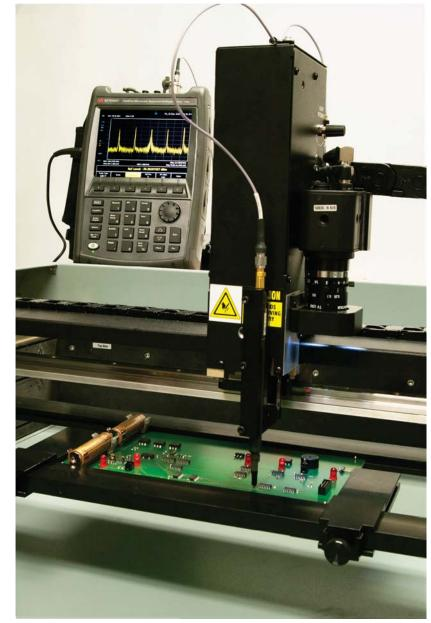
Langer RF-B 3-2 RF Probe fitted to the Access RF Prober. The RF probe is connected to a Keysight N9935A Spectrum Analyzer and is used to measure near field signals on a circuit board.
