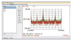
Failed test points are listed in order of severity in the Workstation Troublesheet view. The stored and current measurements are overlaid in contrasting colors for easier analysis.
