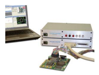
DIP clips and cables, custom cables to PCB connectors or interface to a bed-of-nails. You can compare one component with another in real-time (64 pins max.) or use your PC to automate testing and scan up to 128 pins.
