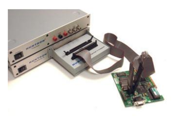
Optional accessories for the Scanners include a connection adapter and IC clip kits. These accessories assist in making the connection to your printed circuit boards easier and helping to speed test times. The Scanner II with the Adapter and a SMT clip/cable are shown to the left.
