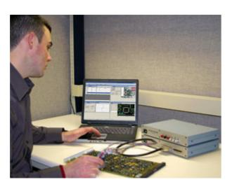
The Huntron Tracker Model 30 is a new compact Tracker designed for use with Huntron Workstation and accessories such as the New Scanner II, the new Scanner 31S or an Huntron Access Prober. Take advantage of Tracker Signature Analysis capabilities to help you troubleshoot printed circuit board (PCB) faults to the component level and without applying power, saving circuits from possible further damage.
