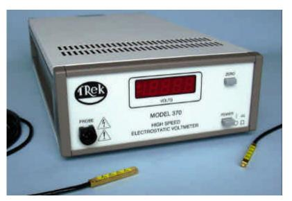
The Trek Model 370 is a precision electrostatic voltmeter with the unique capability of making noncontacting surface voltage measurements in the range of 0 to ±3 kV DC or peak AC.
