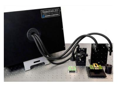
The SpectralLED<sup>®</sup> Fiber Optic Output configuration provides flexible illumination for applications where space is limited. Systems can be configured with multiple outputs enabling several devices to be simultaneously illuminated at different working locations. Collimating optics are included at the fiber distal end, and custom fiber diameters and lengths are available.
