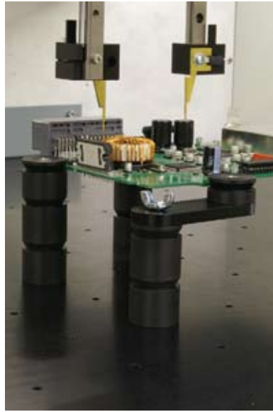
Mounting a PCB in the Access DH using the Rotating Board Holder kit. The pieces can be combined for optimum flexibility.
