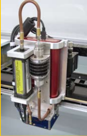
Custom multi-pin probe head for point-to-point RF measurements
