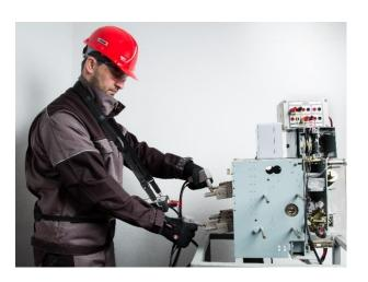
When testing live tank HV circuit breakers with RMO-H a different cables length may be used. The short cable (red cable, 1,3 m) connects the RMO-H to the CB's bushing close to the test person and the device. The long cable (black cable, 3 or 5 m) is connected to a further away positioned bushing on the other side of the breaking point.
