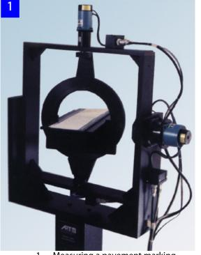
1. Measuring a pavement marking
