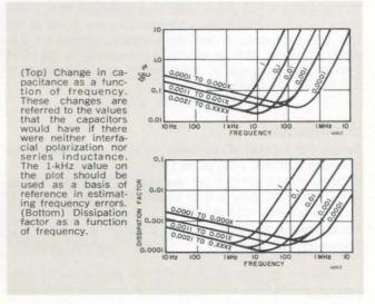
**Dissipation Factor:** Not greater than 0.001, 0.0005, and 0.0003 for capacitances of 100 to 1000 pF, 1100 to 2000 pF, and 2100 pF to 1.1110  $\mu$ F, respectively.
