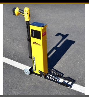
Agencies and contractors require a rapid and efficient way to verify the retroreflectivity of pavement markings. The StripeMaster<sup>®</sup> Touch series is a highly reliable, field-proven tool for safe and consistent measurement values with minimal operator training.
