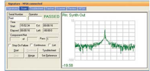
Using the Huntron Workstation SDK, this NFSA signature can be displayed in the Workstation Signature pane
